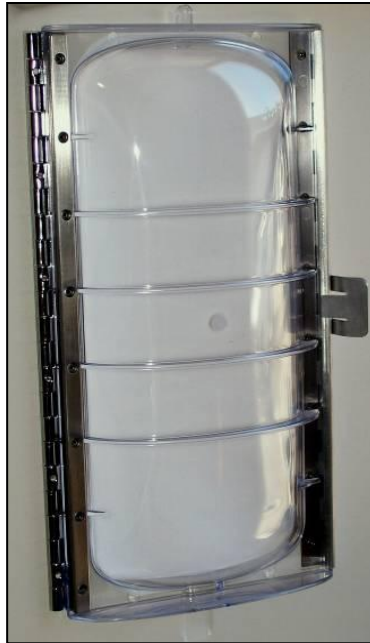
Solution Pressurization Chamber
